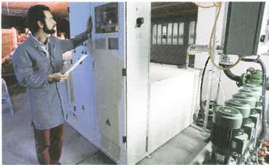
Environmental protection and security: Microscopic tears must be avoided at all costs in solid carbide grinding. This high-volume cooling and micro-filtering plant has been installed in the basement.
