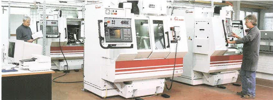
Efficiency: At the new location, nine of these modern CNC form-relieved grinding machines are on line.
